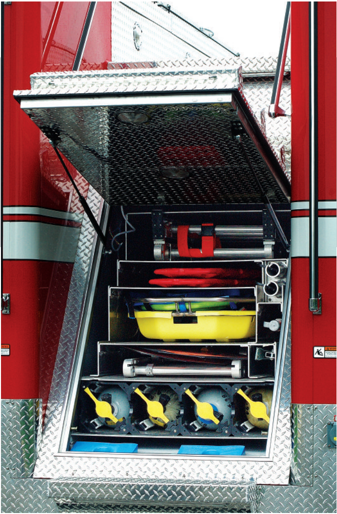
Under staircase storage provides easy access to large, long items. Hidden under the stairs when not in use, these items are ready for immediate access at the release of a single latch.
