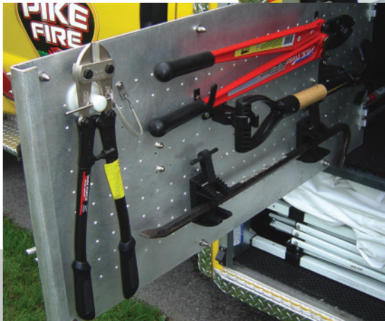
Dedicated storage is specifically designed to accommodate hydraulic rescue tools and equipment.
