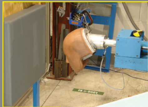
A head-strike cannon was used to test the HOPS cushion system.
